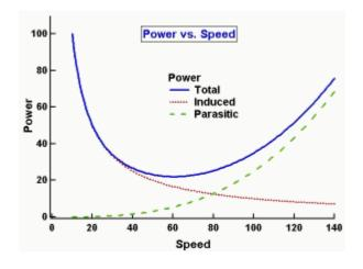
Fig 10 Power requirements versus speed.
