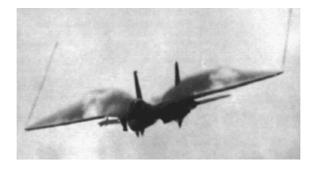
Fig 14 Condensation showing the distribution of lift along a wing. (from Patterns in the Sky, J.F. Campbell and J.R. Chambers, NASA SP-514.)
