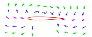
Fig 6 Direction of air movement around a wing as seen by an observer on the ground.
