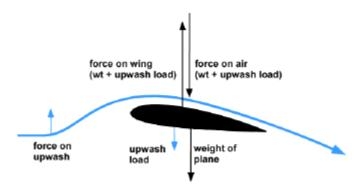
Fig 15 Wing out of ground effect
