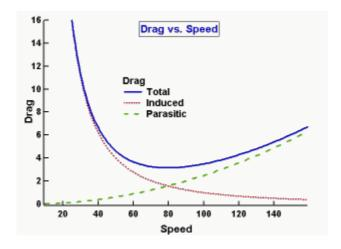
Fig 11 Drag versus speed.
