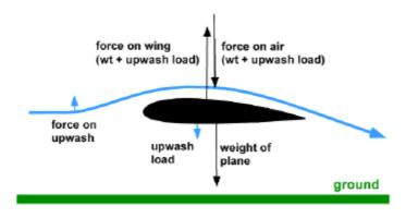
Fig 16 Wing in ground effect
