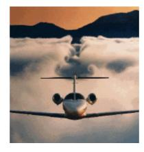
Fig 5 Downwash and wing vortices in the fog. (Photographer Paul Bowen, courtesy of Cessna Aircraft, Co.)
